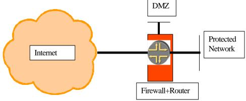
"Internet ↔ firewall/router(edge device) ↔ net" architecture
